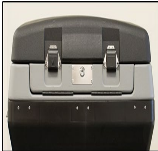
Figure 20 - Unhooked Latches on Scanning Unit
