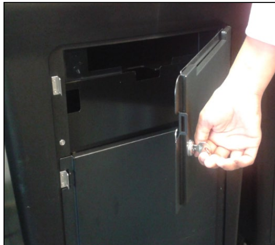
Figure 14 - Opened Emergency Ballot Compartment Door
