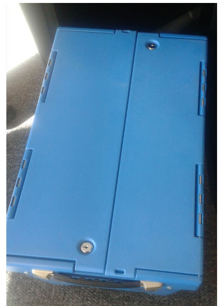
Figure 48 - "Tongue-in-groove" Fit on the Ballot Transfer Bin
